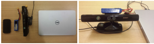
Figure 3: Our experimental setup. Left: components from left to right are a smartphone, battery, Kinect, and laptop. Right: Kinect, phone, and battery fixed together for scanning.
