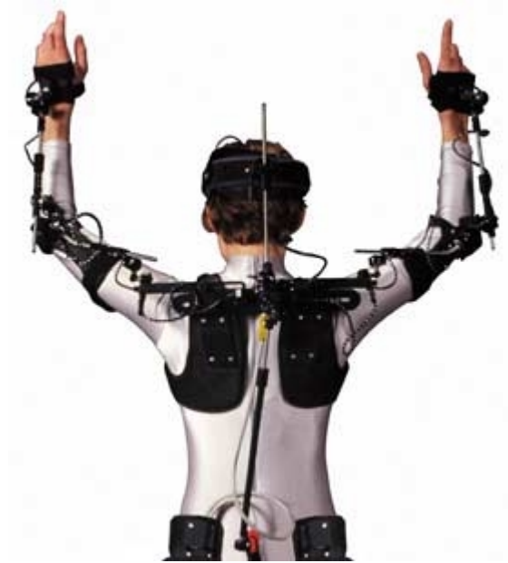
Figure 10 Example exoskeleton based motion capture technology. These systems use a mechanical structure fitted onto the actor's body.
