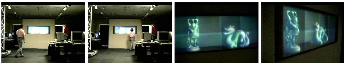
Figure 73 Using the large scale motion recovery sub-system to track a users head position ensures that the correct projection of a virtual object can be rendered on a wall size display.
