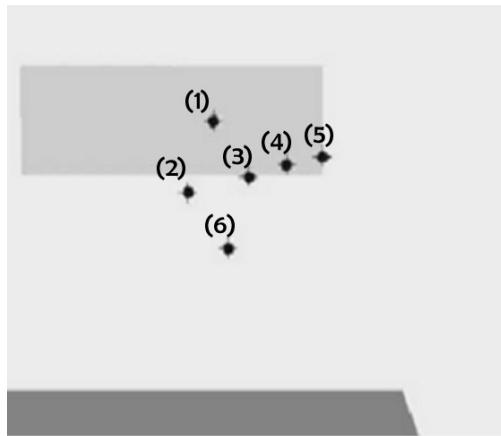
Figure 34 Rather than determining target location separately at each time instant, a motion model can be used to maintain an estimate of target location. One of the benefits of using a motion model is that consistent target IDs can be maintained. Here we see target locations with their associated IDs.
