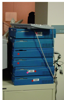
Figure 22 (Left) Cameras are connected to machines through a patch panel in order to provide configuration flexibility. (Right) The stacks of Indy's shown here, as well as Wintel PCs, are used to digitize video and locate features.
