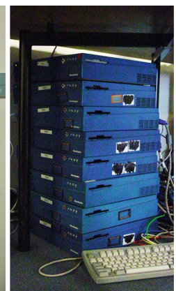
Figure 22 (Left) Cameras are connected to machines through a patch panel in order to provide configuration flexibility. (Right) The stacks of Indy's shown here, as well as Wintel PCs, are used to digitize video and locate features.
