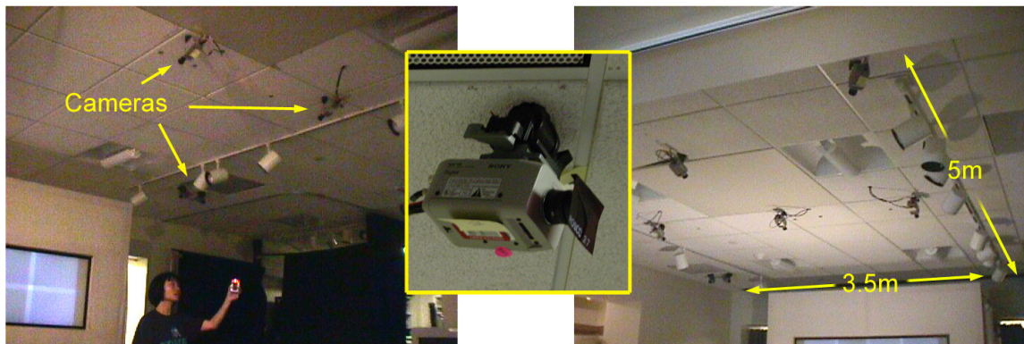
Figure 18 Cameras mounted on the ceiling of a laboratory are used to capture large scale motion.
