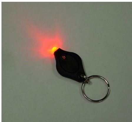
Figure 19 An LED light source is a useful feature to track, since detecting it against a wide variety of backgrounds is easy and robust.
