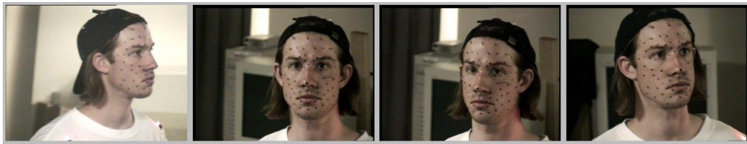
Figure 54 The view from each of the four pan-tilt cameras. The cameras all look at the same point, but provide images from different angles, allowing triangulation of features.
