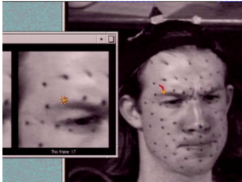
Figure 55 Video figure The small scale recovery system uses painted marks as features for motion recovery. A close-up of features on the face is shown here.
