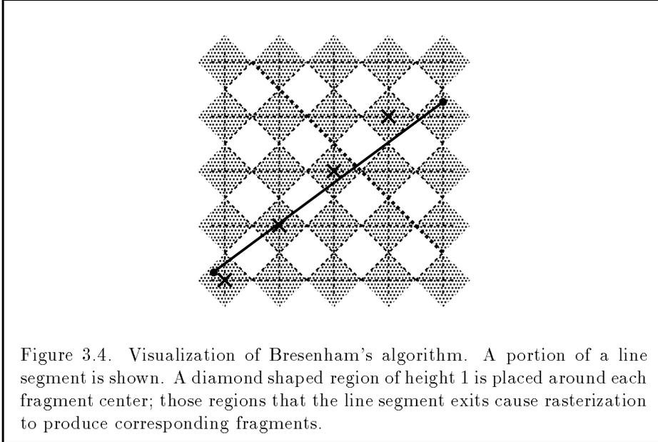
Figure 3.4. Visualization of Bresenham's algorithm. A portion of a line segment is shown. A diamond shaped region of height 1 is placed around each fragment center; those regions that the line segment exits cause rasterization to produce corresponding fragments.
