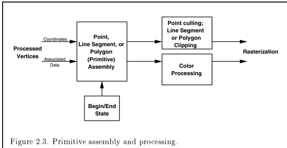
Figure 2.3. Primitive assembly and processing.
