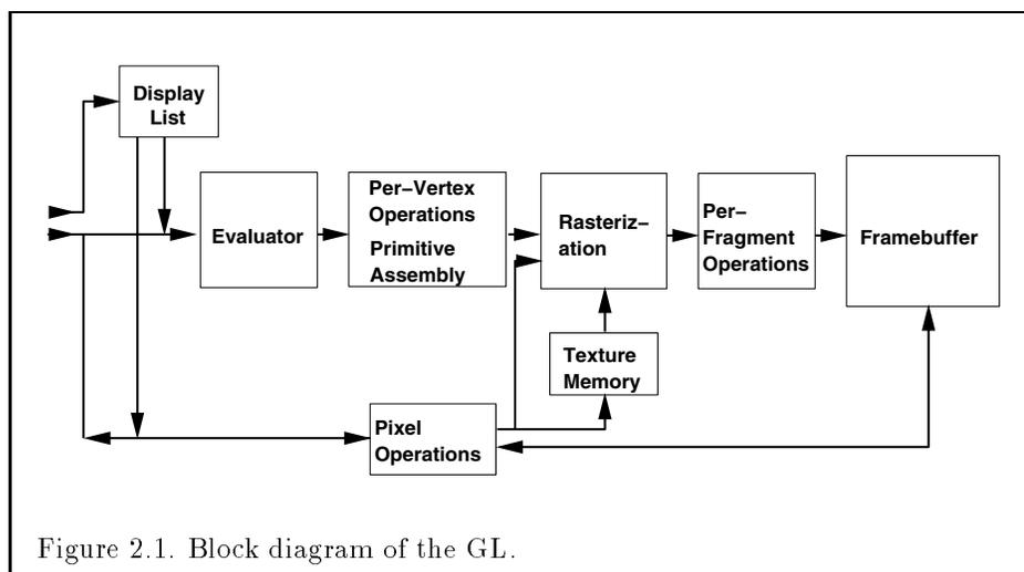
Figure 2.1. Block diagram of the GL.
