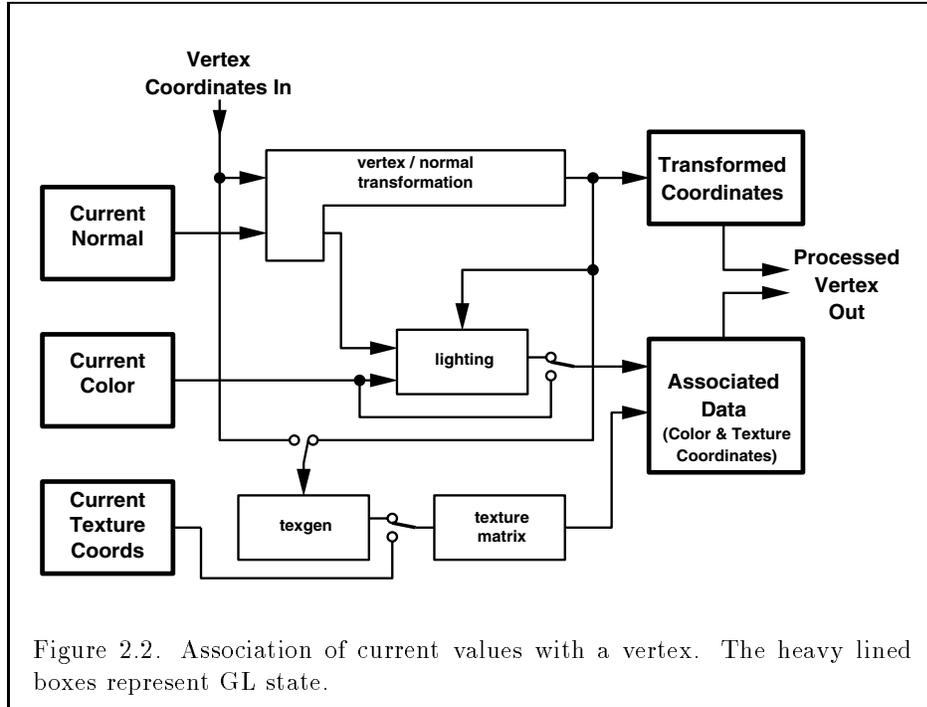
Figure 2.2. Association of current values with a vertex. The heavy lined boxes represent GL state.
