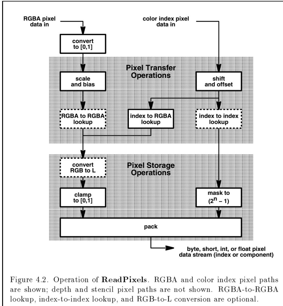
Figure 4.2. Operation of `ReadPixels`. RGB and color index pixel paths are shown; depth and stencil pixel paths are not shown. RGB-to-RGB lookup, index-to-index lookup, and RGB-to-L conversion are optional.
