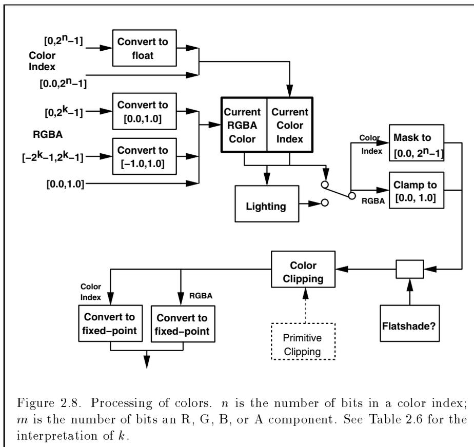
Figure 2.8. Processing of colors.  $n$  is the number of bits in a color index;  $m$  is the number of bits an R, G, B, or A component. See Table 2.6 for the interpretation of  $k$ .
